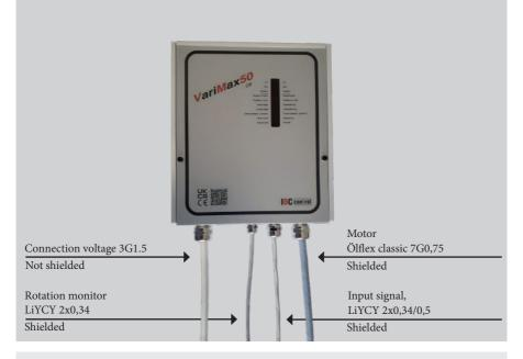
EMC glands must be used for shielded cables. The above cables or equivalent must be used to comply with the EMC Directive.
