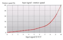
The input signal is directly proportional to the efficiency of the rotor, which means that input signal and rotation speed are as per adjoining diagram.
